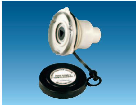
CLF-07 Polypropylene female Clean-Lock, container portion with 2 in (50 mm) buttress threads and EPDM tank gasket. Includes an O-ring on the built-in check valve preventing any air leaks or tank cross contamination.
