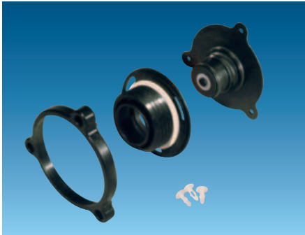
Vent-00 Tamper evident 2 in (50 mm) buttress vent with EPDM tank gasket, Viton® O-rings and plastic rivets for tamper evident seal. Vent-01 Tamper evident 2 in (50 mm) NPS vent with EPDM tank gasket, Viton O-rings and plastic rivets for tamper evident seal.
