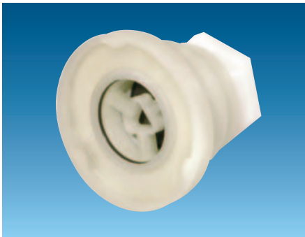
CA ASSY Clean Aid assembly for male Clean-Lock. A one-way valve is built into each Clean Aid to prevent back flow into clean, uncontaminated rinse water. Note: Clean Aid should not be used as tank coupler.
